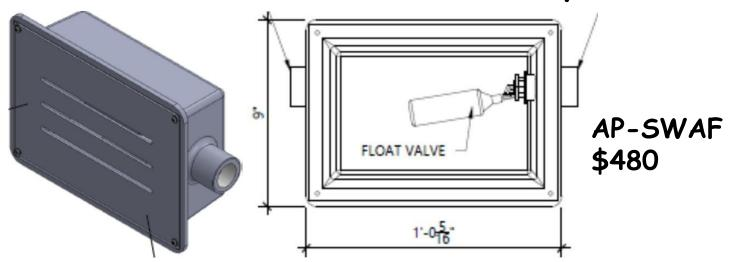
Fiberglass body Plastic front plate BLACK float valve assy, 1" fresh water, 1" overflow
