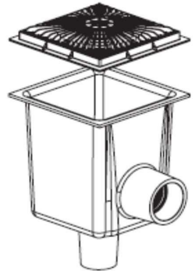
Main Drain Sumps
